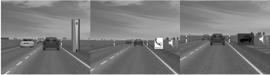
Fig.1. Info-Assistant, visual feedback of the Warning-Assistant and visual feedback of the Brake-Assistant, trial with clear visibility
