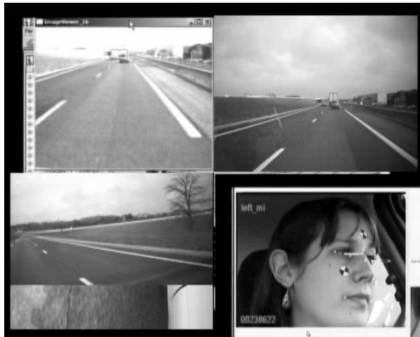
Fig.1. Video sources from: stereo-vision camera with radar for distance estimation to obstacles (top left), the front view (top right), the rear view (down left – upper part), the view from the left outside mirror down to the surface of the road (down left – lower part), and the view to the participants head with the glance direction of the eye (down right)
