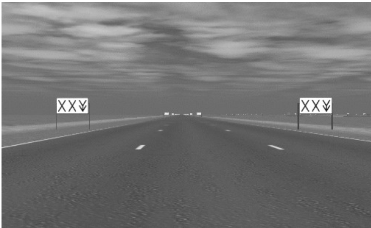
Fig.2. Screen shot from the LCT. In this instance the driver has to change from the centre lane to the right lane.
